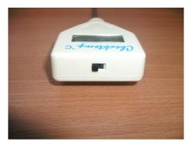
After switching on, the temperature should be displayed on the screen (if this does not happen, the battery may require changing)
